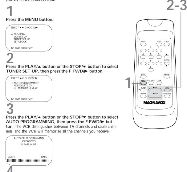
Wait for a few minutes while the VCR sets up the channels. When this is complete, CHANNELS ARE SET will appear on the screen. Then the programming of the lowest channel number placed in the VCR's memory will appear on the screen. Now when you press the CHANNEL ▲/▼ buttons, you will scan only through channels you receive.
